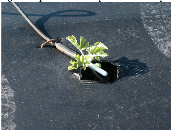
Fig 1. Temperature sensor placement in crop canopy.
