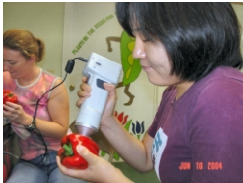
Photo 4. Using a Minolta Chroma Meter (CR-200) to measure color parameters.
